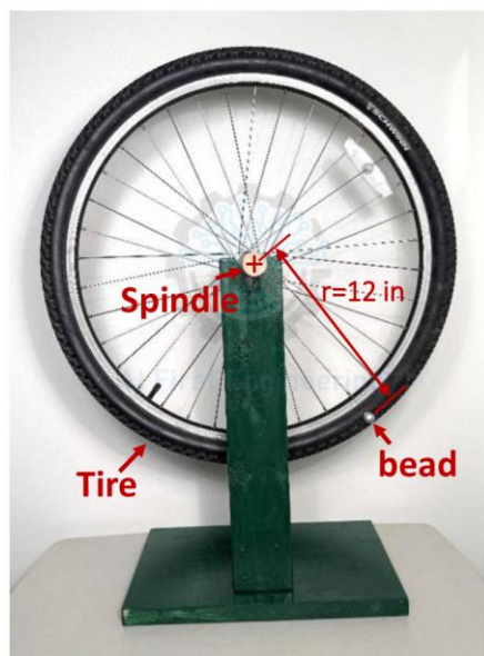
Figure A1 — bicycle-wheel apparatus: spindle, tire, and the bead at r \approx 12\text{ in} from the spindle center.
